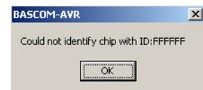
Check your cable and refer to the troubleshooting procedures at the end of this manual. When you get into the programmer, click on the Autoprogram button in the toolbar. This button looks like a green IC with a T next to where pin 1 would be. This will transfer your program to the Mega48 and then read the program back out of the chip to verify that it got programmed correctly.
