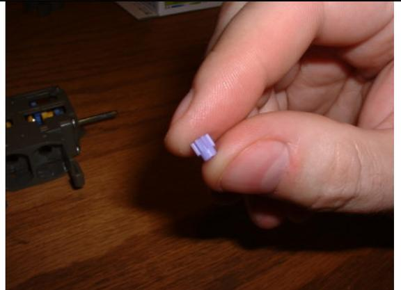
Place the G1 gear on end of each motor shaft as shown in the photo. Slide it far enough on that it stays in place.
