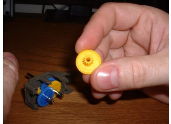
Place the yellow G2 gear onto the hex shaft as shown in the picture. The small gear on the G2 should mesh with the larger gear on the G3
