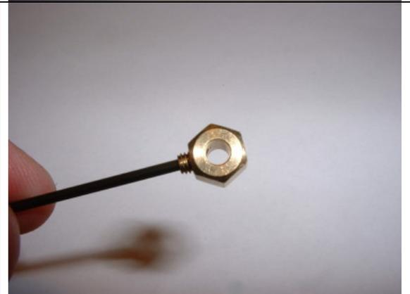
Now slide the gear hub onto the hex shaft. If the hub won't slide on, back out the set screw until it does. Snug the screw slightly but don't tighten it yet.
