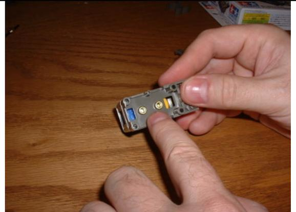
Locate the right side housing part (should be the last part left) and the last 2 brass eyelets. Place the eyelets into the holes as shown in the picture.
