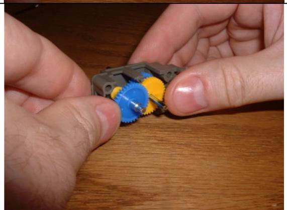
Find the yellow G2 gear. This gear has teeth on the face instead of the edge.
