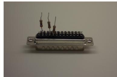
*Solder three resistors to connector.*
