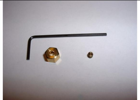
The set screw is very small. to make it easier to install the set screw into the gear hub, place it on the end of the hex wrench as shown in the picture.
