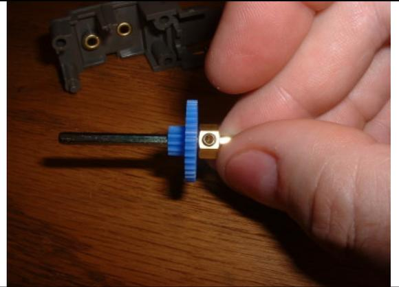
Slide the hex shaft into the right hole as shown. The short side of the 2 axles should now be about lined up with each other.
