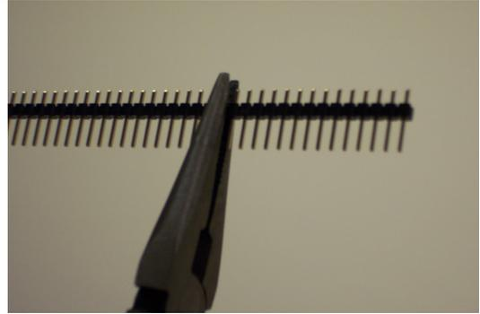
Take one of the 40-pin headers and snap off two 14-pin headers and two 5-pin headers. These will be for J1 and the two power headers for ground and +5V. One pad for each power trace will be wired to the breadboard. From the other 40-pin header, snap off one 5-pin header for J3, the programming header. Snap off another three 4-pin headers for J7 and J8. Finally, snap off one 2-pin header for J9. This will enable or disable the motor driver chip.
