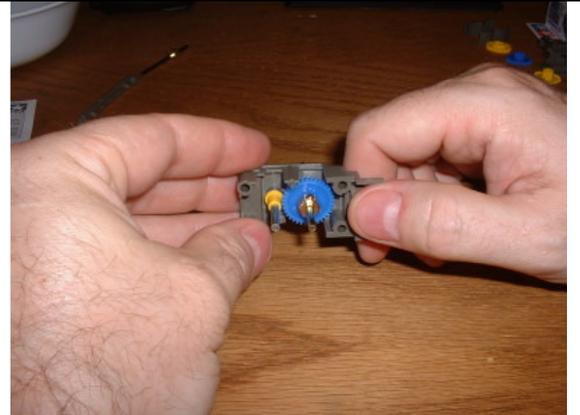
Find the yellow G4 gear, it has a hex shaped protrusion on one side that will fit onto the gear hub on the hex axle.
