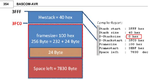
Picture: SRAM for example with h = 64, s = 64, s = 0, f = 256
