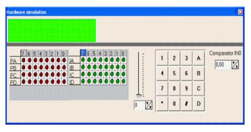
The top section is a virtual LCD display. It works to display code in PIN mode, and bus mode. For bus mode, only the 8-bit bus mode is supported by the simulator.
