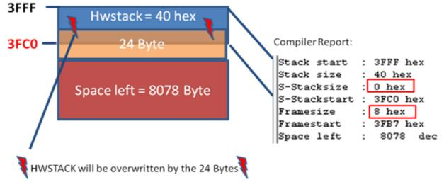
Picture : SRAM for example with = 64, swstack = 0, framesize = 8
