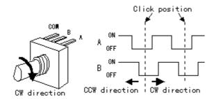
Since the microprocessor has internal pull up resistors, you do not need external pull up resistors for most encoders.
