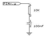
The capacitor is charged and the time it takes to discharge it is measured and stored in the variable. Now when you vary either the resistor or the capacitor, different values will be returned. This function is intended to return a relative position of a resistor wiper, not to return the value of the resistor. But with some calculations it can be retrieved.
