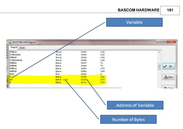
Picture: How to see which Variables are stored on which SRAM Address
