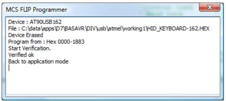
The FLIP programmer window will be closed automatic when the programming succeeds.
