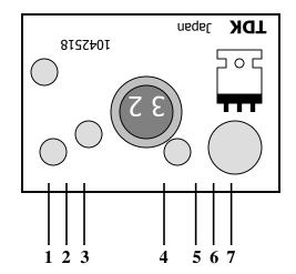
The TDK 1042518 is ideal for portable devices that are powered by 2-4 cells or by a single Li-Ion/Li-Poly battery. It outputs a stable +5v up to 250ma and -5v up to 70mA.
